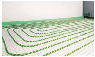
To enable the **PRINETO** Velcro surface heating pipe to be fixed onto the high-quality sound insulation and heat insulation boards, these have Velcro fleece laminated onto their surface. In conjunction with foil overlap on the long sides, adhesive strips ensure the lengths are bonded screed-tight.
