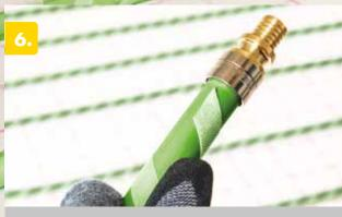
For the manifold connection or pipe connections, unwind about 5 cm Velcro tape at the end of the heating pipe and cut this off using a sharp blade
