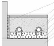
Edge insulating strip Flooring Heated screed U. heating pipe 14, 17, Stabil 16x2,0 Tacker foil Thermal- and sound insulation Diffusion barrier (optional) Raw floor
