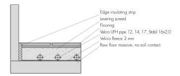
This floor structure is only possible with special screeds listed below with a minimum system coverage.
