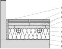
Edge insulation strip Flooring Dry elements Special glue (optional) Aluminium foil UFH pipe Stabil 16x2,0 EPS-element Diffusion barrier (optional) Raw floor
