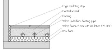
This floor structure is only possible with special screeds listed below with a minimum system coverage.
