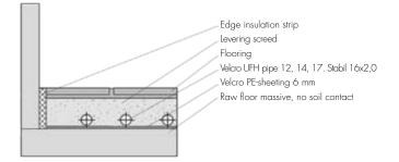
This floor structure is only possible with special screeds listed below with a minimum system coverage.
