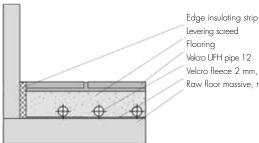
Velcro UFH pipe 12 Velcro fleece 2 mm, perforated Raw floor massive, no sail contact
