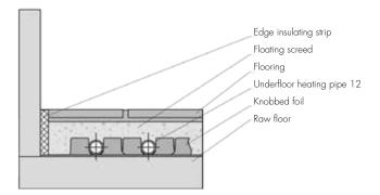
Installation only in combination with a load-bearing surface and with leveling screed.
